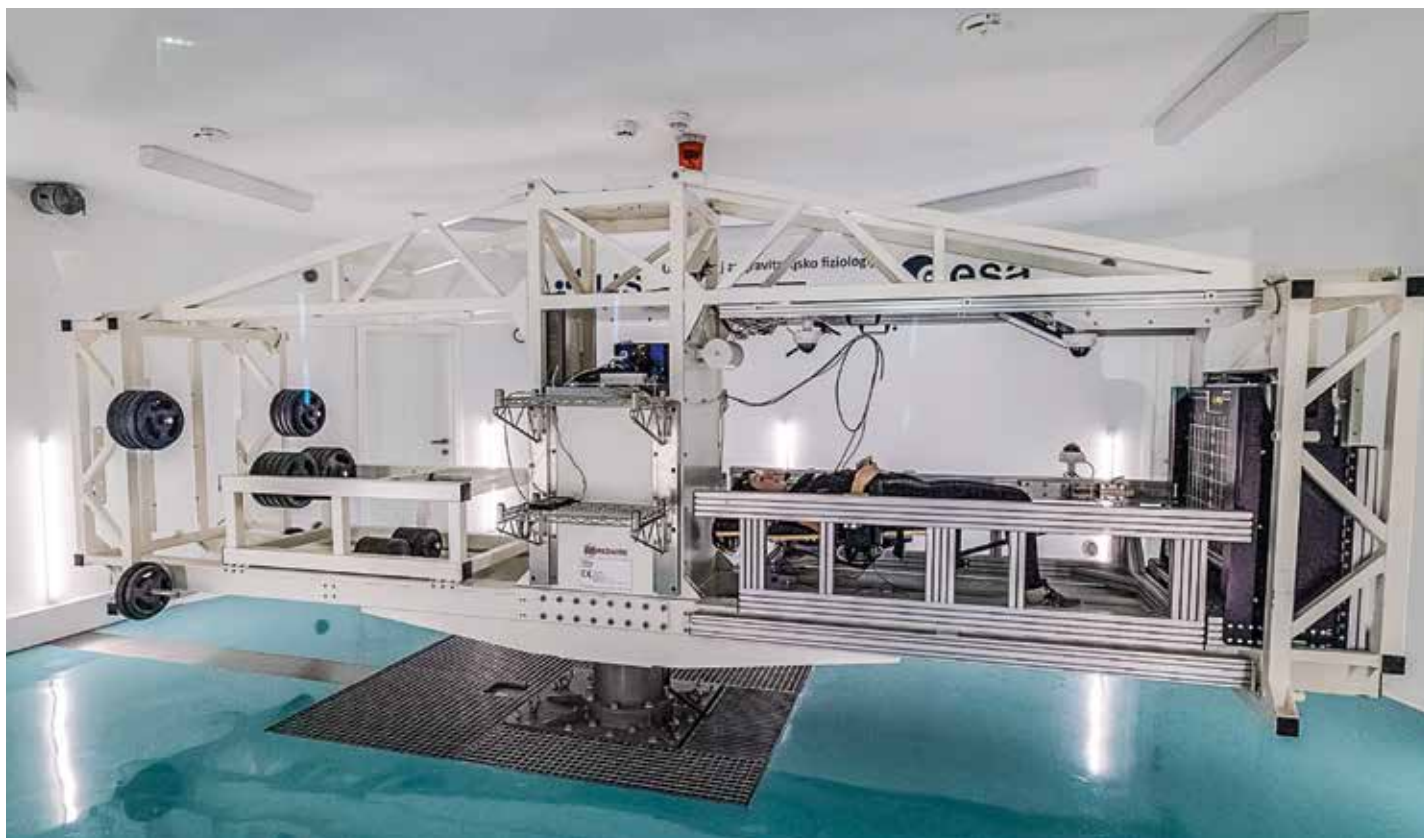
The human centrifuge at the Planica Nordic Centre is an advanced research facility for studying the effects of artificial gravity and simulated space conditions on the human body. Photo: Marjan Verč
