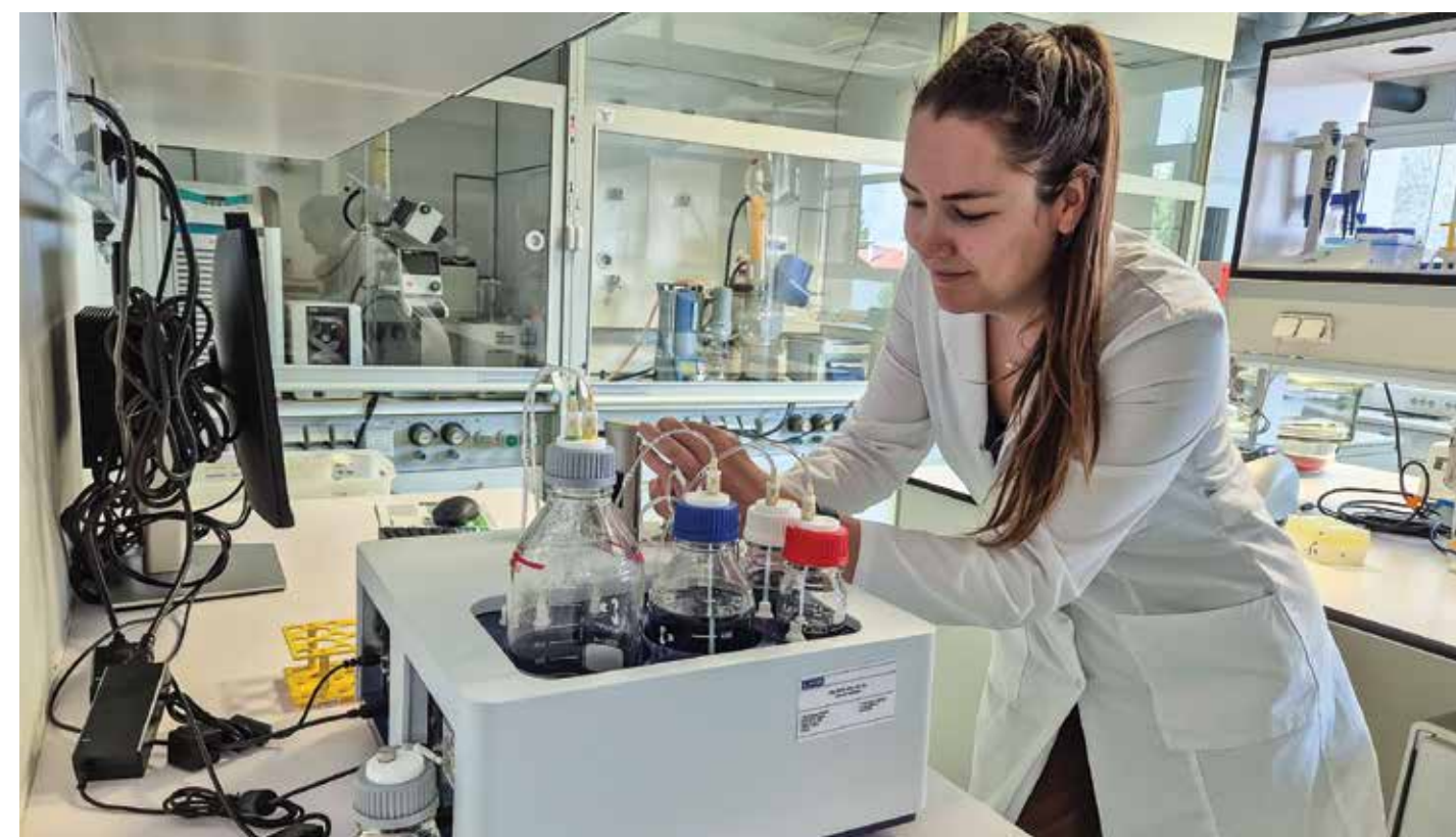
An isothermal titration calorimeter enables researchers at the National Institute of Chemistry to study the interactions between proteins, nucleic acids and other biomolecules. Photo: Archive of the National Institute of Chemistry
