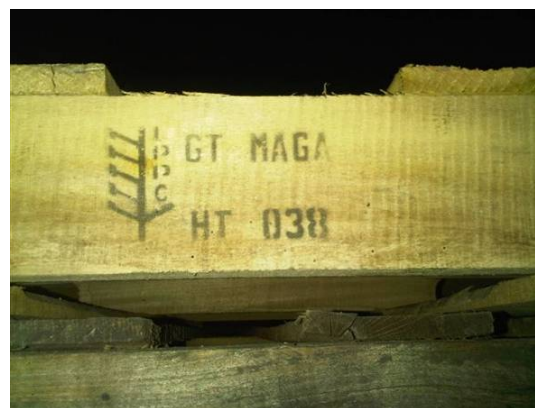
Figure 4 6 – Mark does not contain the required borders.
