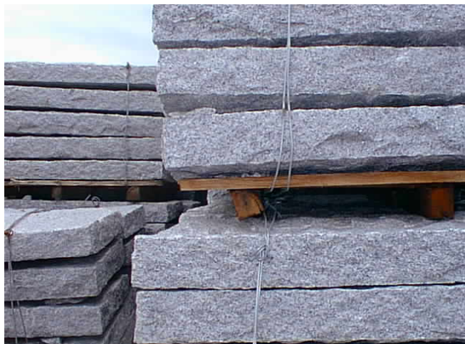
Figure 5 - Dunnage attached to stone shipments
