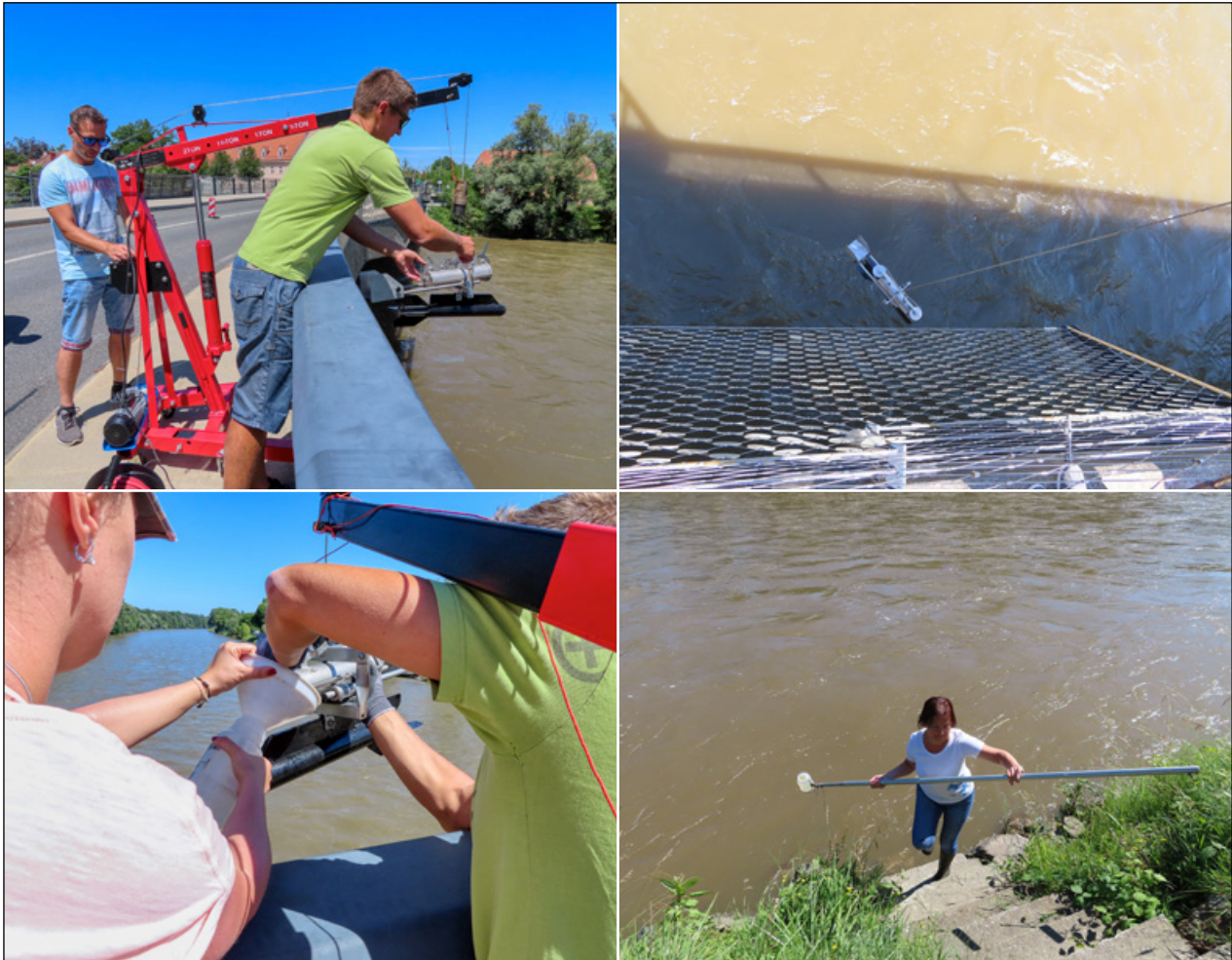
Slika 4: Izvajanje profilne meritve suspendiranih snovi (vir: Arhiv ARSO) Figure 4: Implementation of profile measurement of suspended solids (Source: ARSO Archives)
