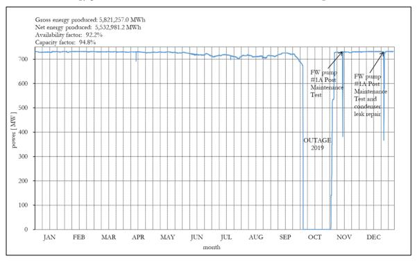
Figure 1: Operating power diagram of Krško NPP in 2019
