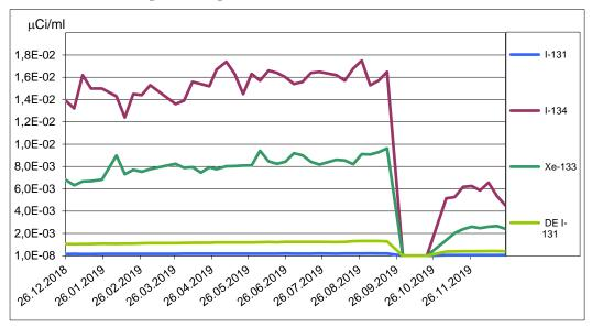
Figure 6: Primary coolant-specific activity – 30<sup>th</sup> and 31<sup>st</sup> fuel cycles
