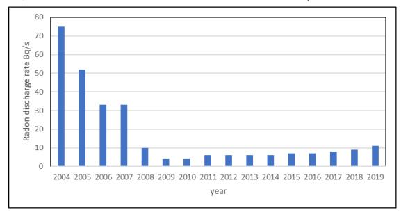
Figure 23: <sup>222</sup>Rn emissions from the Central Radioactive Waste Storage Facility in Brinje
