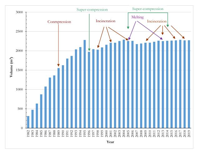
Figure 25: The accumulation of low- and intermediate-level radioactive waste in the Krško NPP storage
