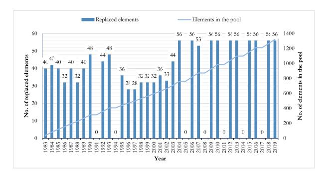
Figure 26: The number of annually spent fuel assemblies and the total number of such elements in the pool of the Krško NPP
