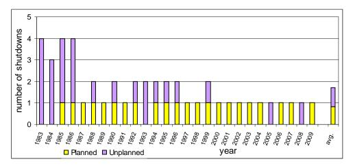
Figure 3: Normal reactor shutdowns – planned and unplanned
