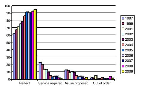
**Figure 16:** Percentage of diagnostic X-ray devices according to their quality for the period 1997–2009
