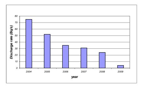
**Figure 18:** Emission rate of <sup>222</sup>Rn from the Central Storage of Radioactive Waste at Brinje
