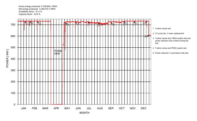
Figure 1: Operating power diagram for the Krško NPP in 2009
