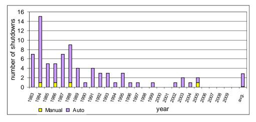
Figure 2: Fast reactor shutdowns – manual and automatic
