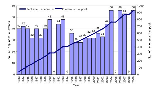
**Figure 21:** The annual production of spent assemblies and accumulation of spent fuel assemblies in the Krško NPP spent fuel pool
