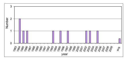
Figure 4: Number of unplanned safety injection system actuations
