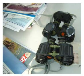
**Figure 12:** Binoculars with <sup>3</sup>H of 37 GBq i.e. well above exemption level of 1 GBq
