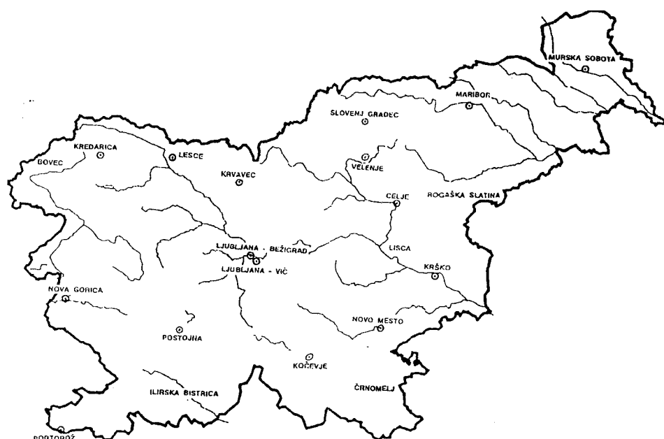
Figure 17. Locations of ROS gamma monitors on meteorological stations. Sign ⊙ marks monitors in operation, locations without signs are planned.
