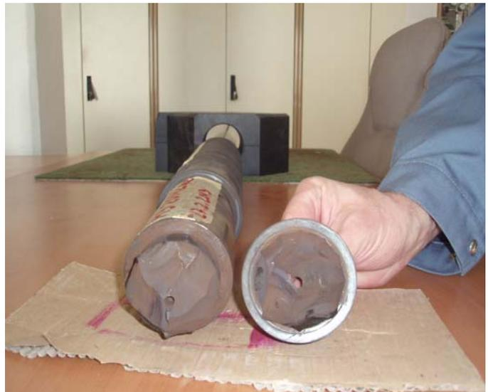
Fig. 1: The broken stem of the main steam line valve
