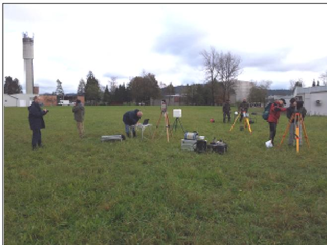
The first set of measurements consisted of dose-rate measurements, which are the first measurements conducted in the event of a radiological or nuclear accident. For this purpose, each team tested several instruments with a calibration source that was placed in the field. Measurements were performed at three distances providing results at different dose rates.
