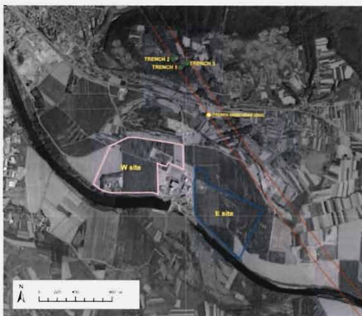
Fig. 1 : Location of trenches on the Libna Hill with respect to the Libna fault (two lines indicate the approximated width of the fault zone) and the two proposed sites. The trench at Stari Grad (reported in 2008) is also shown.
