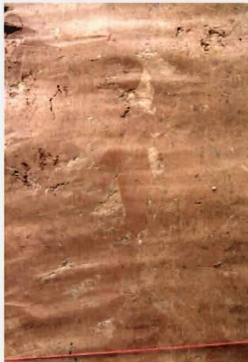
Fig. 38. Cavities that formed along the fractures are filled by silt. NE wall of the Trench 2 at 11.6 m.
