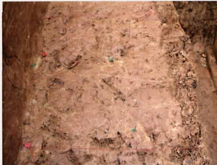
Fig. 36. A net of differently striking fractures along which the “residual clay” is more pale colored or even greenish grey. The fractures dip mostly to the NE. Step of the trench from 3 m to 4 m.
