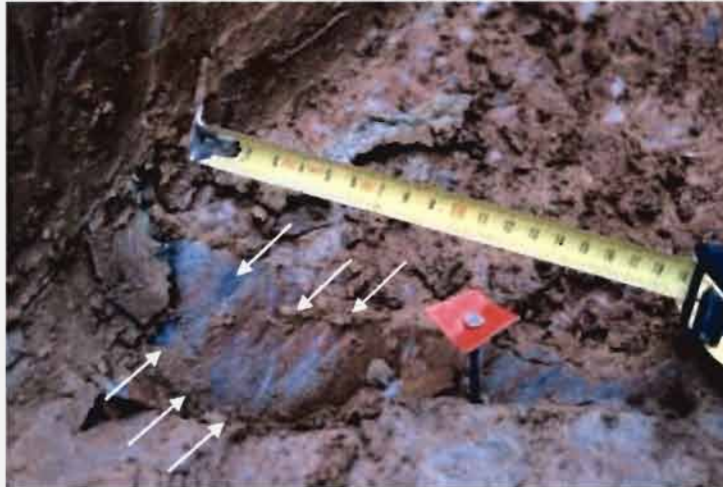
Fig. 26. Horizontal and gently dipping striations are found within the Plioquaternary succession (fault plane : N135, 55°E, striae plunge : 37°S, dextral)
