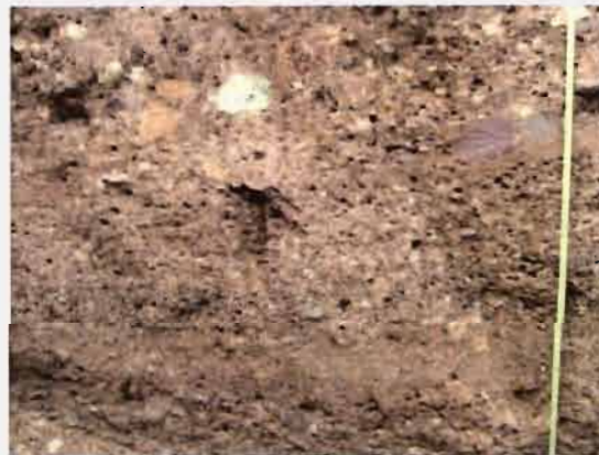
Fig. 13 Larger clasts are oriented with long axis parallel to the lower bedding plane in the lower part of the Unit 5. A fracture filled by silt. The NE wall of the Trench 2, around 22 m.
