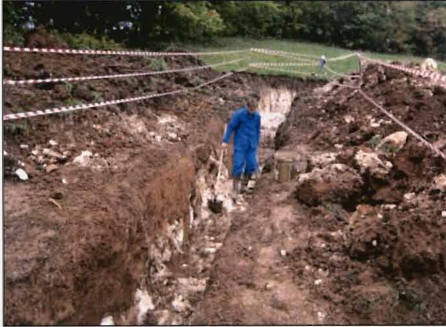
Fig. 7 Badenian limestone is covered by the “residual clay”, while at the WSW tip (trench back, behind the man) of the trench it is covered only by a recent soil.
