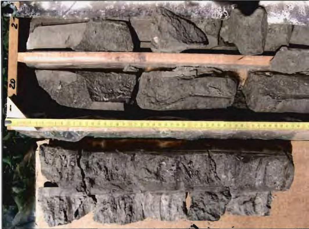
Figure 71: Laminated muscovite carbonate silt in the interval 19.5-20m drilled with diameter 76mm and massive muscovite carbonate silt in the interval 20.0-20.5m drilled with diameter 101mm, ES-2.
