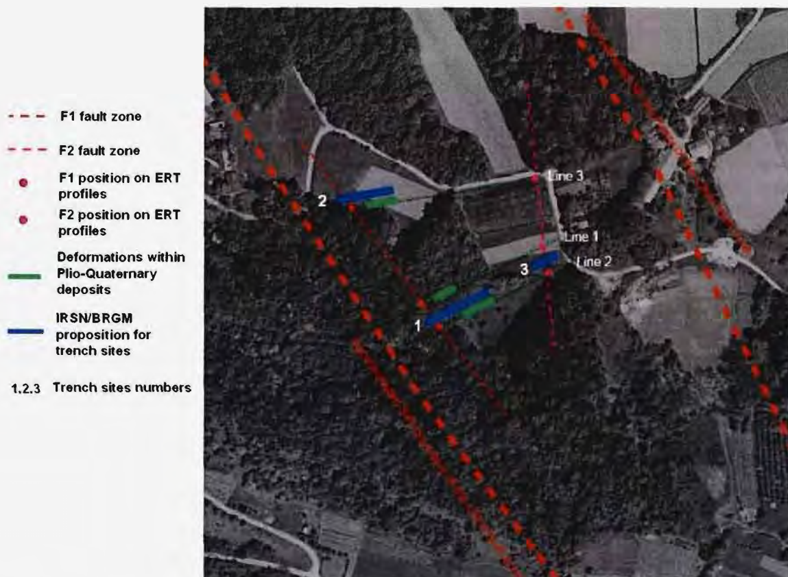
Figure 60. Location of ERT lines (lines 1 to 3), principal structures observed on ERT and proposed trench sites
