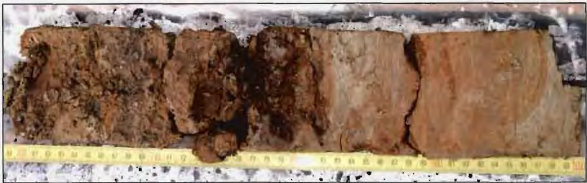
Figure 76: The disconformity at 63.60m between the oxidized Miocene (Pliocene) muscovite carbonate silt and Plio-quaternary polymict silty sandy gravel. ED-1.
