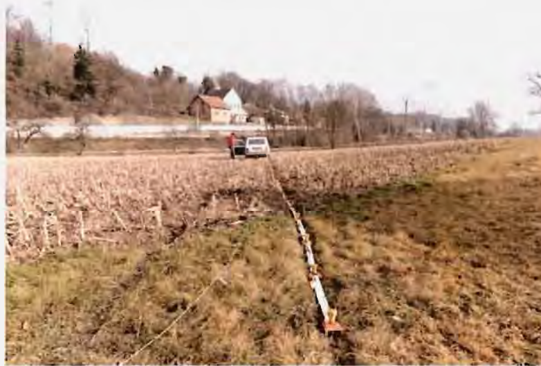
Figure 42. “Landstreamer” acquisition setup for seismic survey across the Libna fault zone
