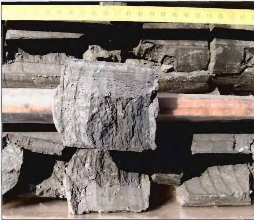
Figure 67: Thin bed (5cm) and laminas of clayey silt in the muscovite carbonate silt. The laminas are horizontal, slightly convex bended on the edges of the core. WD-1, 16.37-16.46m.
