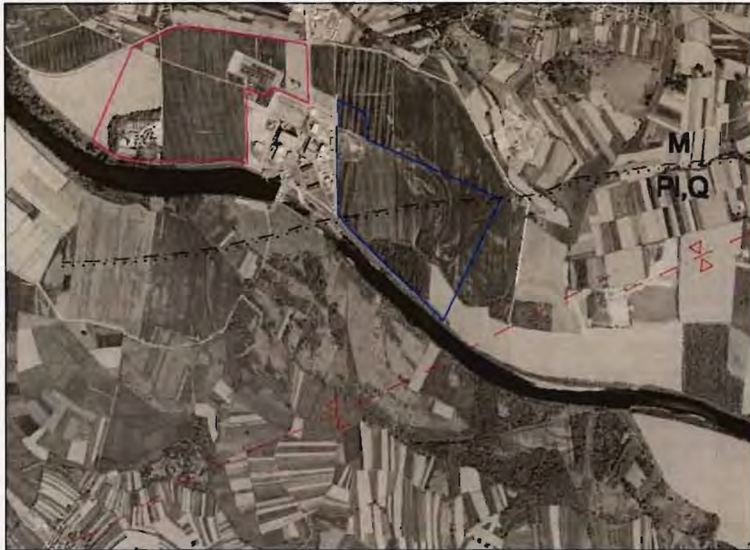
Figure 64. Approximated pinch out line (black dashed) of the Plioquaternary (M/PIQ boundary) underneath the Holocene gravel cover. Plioquaternary sediments fill the central part of the Krško syncline (red dashed) South of the line.
