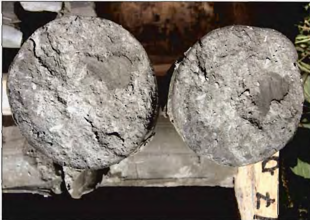
Figure 70: On the convex parting plain circle orientation marks can be observed. ES-2, 17.95m.
