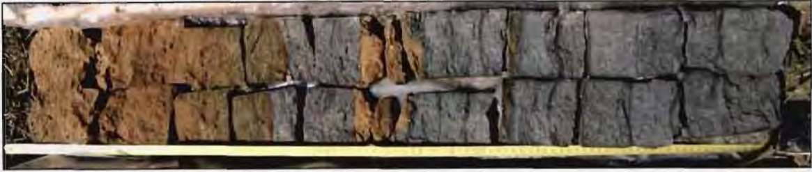
Figure 75: Near the disconformity the muscovite carbonate silt, sandy silt and very fine sand were oxidized and are colored brown. ED-1, 65.0-66.0m.
