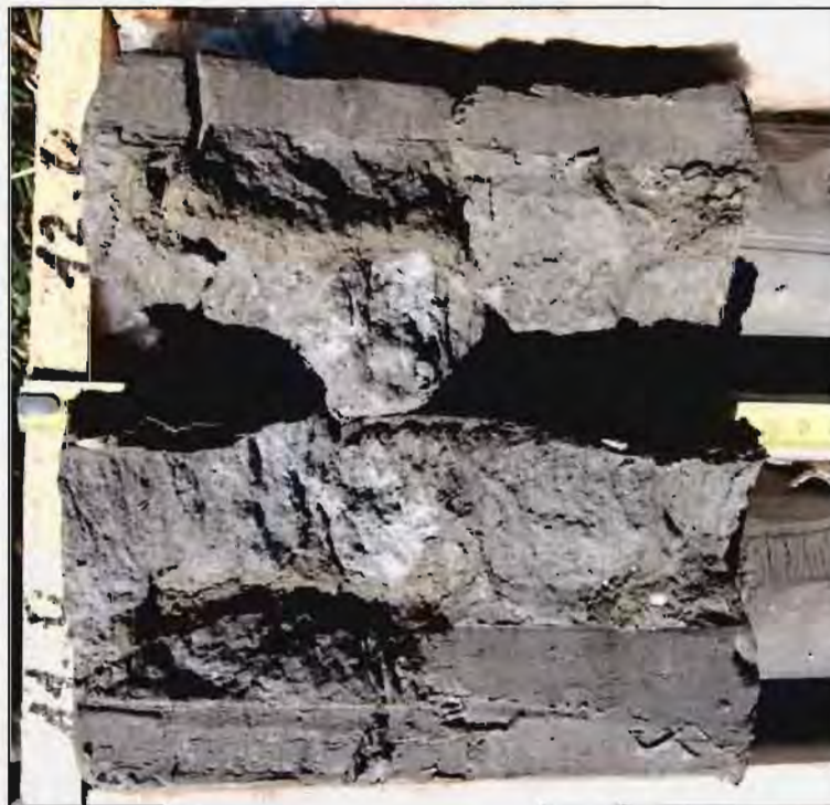
Figure 71: Laminated muscovite carbonate silt in the interval 19.5-20m drilled with diameter 76mm and massive muscovite carbonate silt in the interval 20.0-20.5m drilled with diameter 101mm, ES-2.
