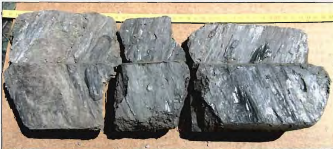
Figure 74: Nearly vertical ( 85^\circ ) tectonic structures produced by oblique-slip movements. ES-2, 33.80-34.20m.
