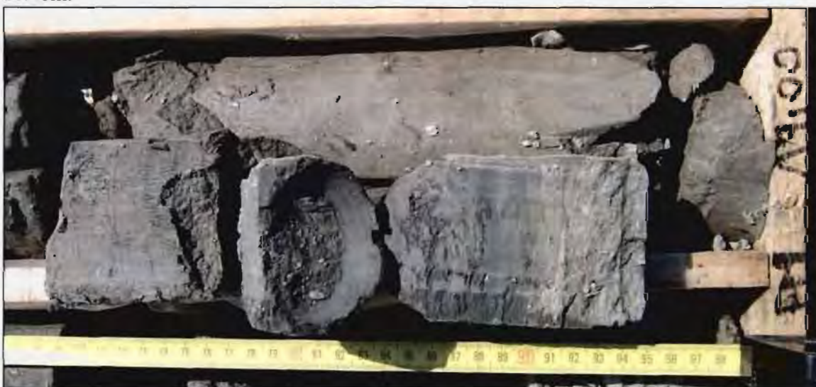
Figure 67: Thin bed (5cm) and laminas of clayey silt in the muscovite carbonate silt. The laminas are horizontal, slightly convex bended on the edges of the core. WD-1, 16.37-16.46m.
