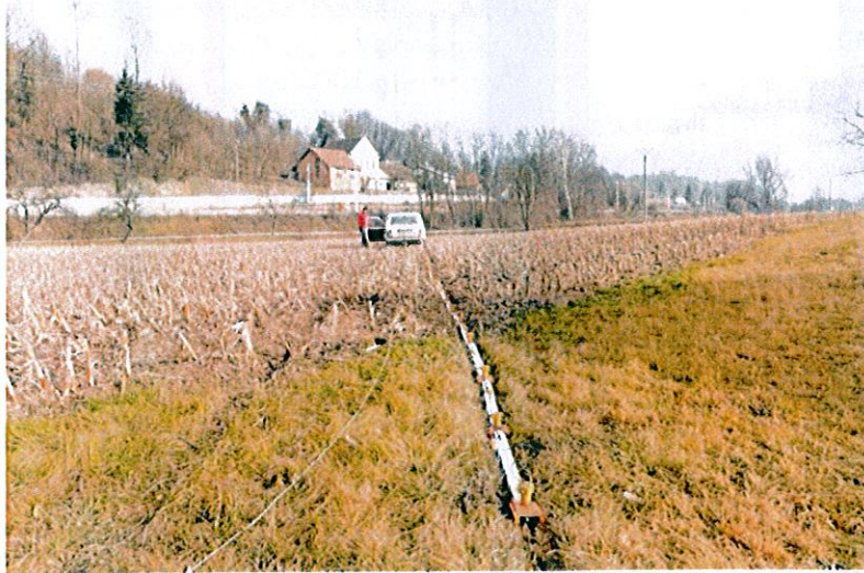
Figure 6. "Landstreamer" acquisition setup for seismic survey across the Libna fault zone
