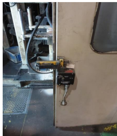
Figure 6: Unscrewed - bypassed safety lock - enabled access to the inside of the machine
