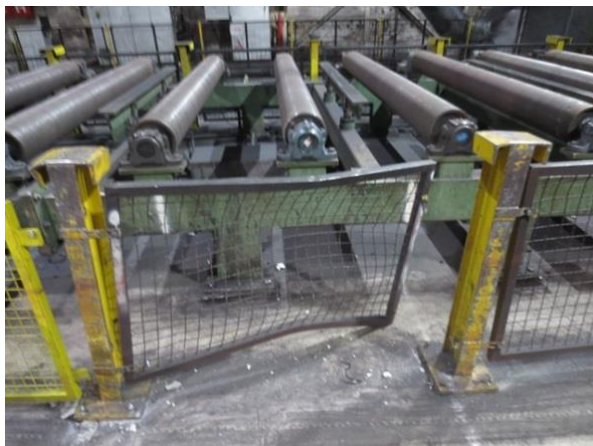
Figure 7: Unscrewed - bypassed safety lock - enabled access to the inside of the machine
