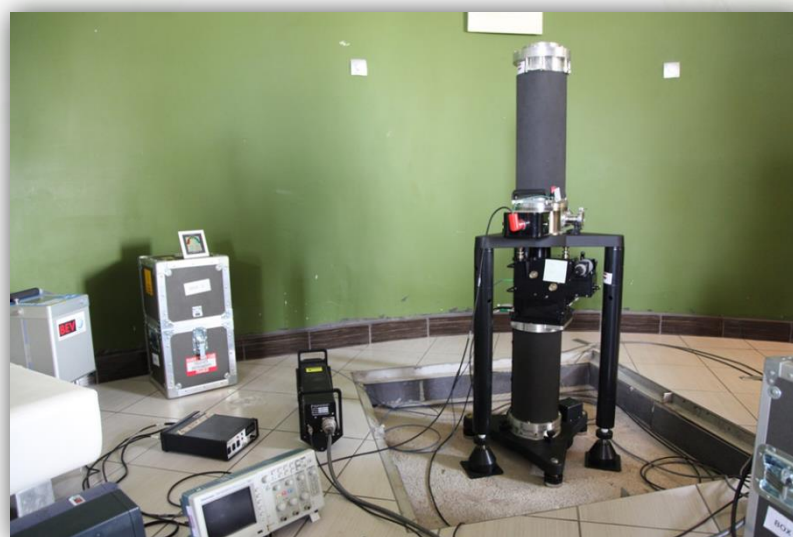
Figure 23: Absolute gravimetric measurements on the AGT300 point in Sevnica
