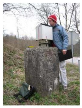
Picture 24: Gravimetric measurement on repers
