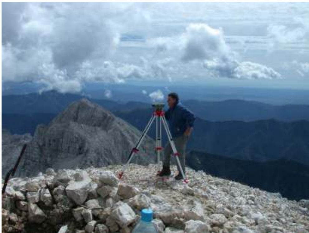
Figure 8: Implementing surveys for determining transformational parameters(photo: Jože Miklič)
