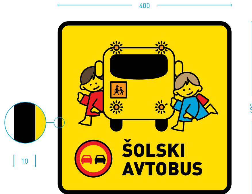
Sign design 2 and sign structure
