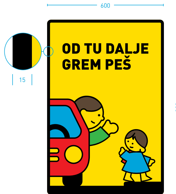
Sign design 3 and sign structure
