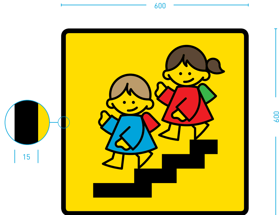
Sign design 2 and sign structure
