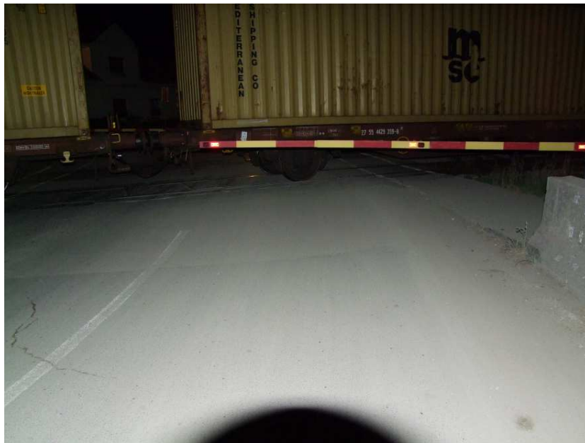
Figure 3: Half-barrier at Vnanje Gorice level crossing reaches as far as the illustrated point
