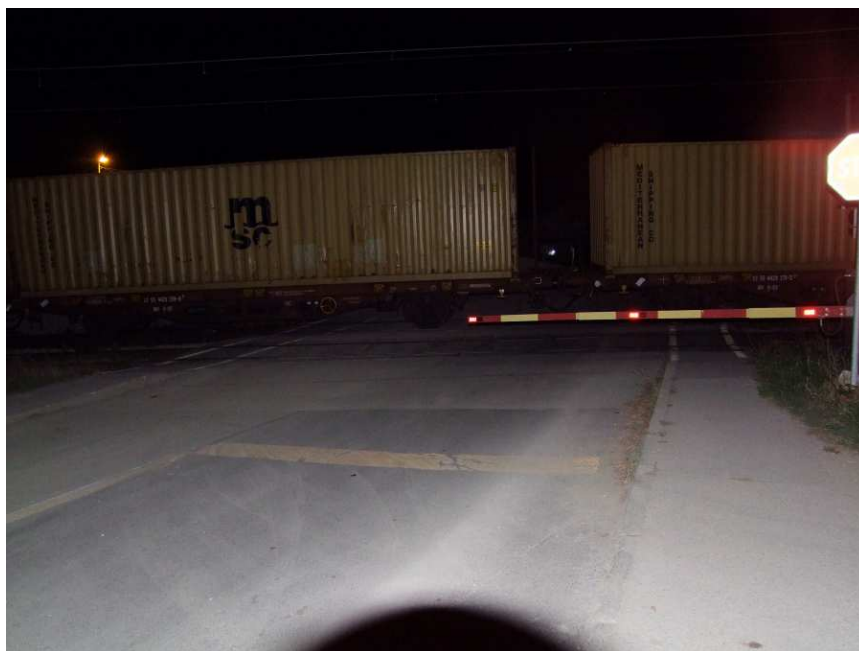
Figure 2: Functioning of the device for protection of the level crossing immediately after the accident when the train involved in the accident was still standing on the level crossing and the consequences of the accident were being removed.
