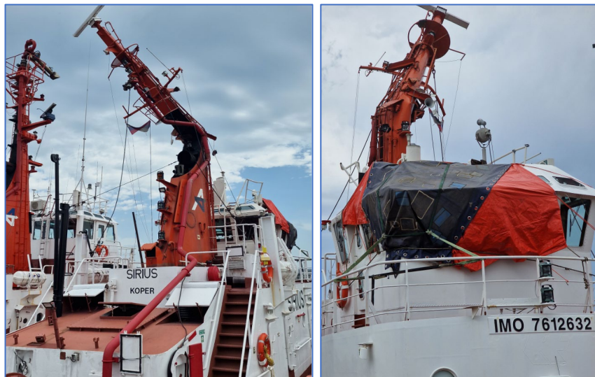
Figure7: Tugboat Sirius - damage to the bridge and main mast.
