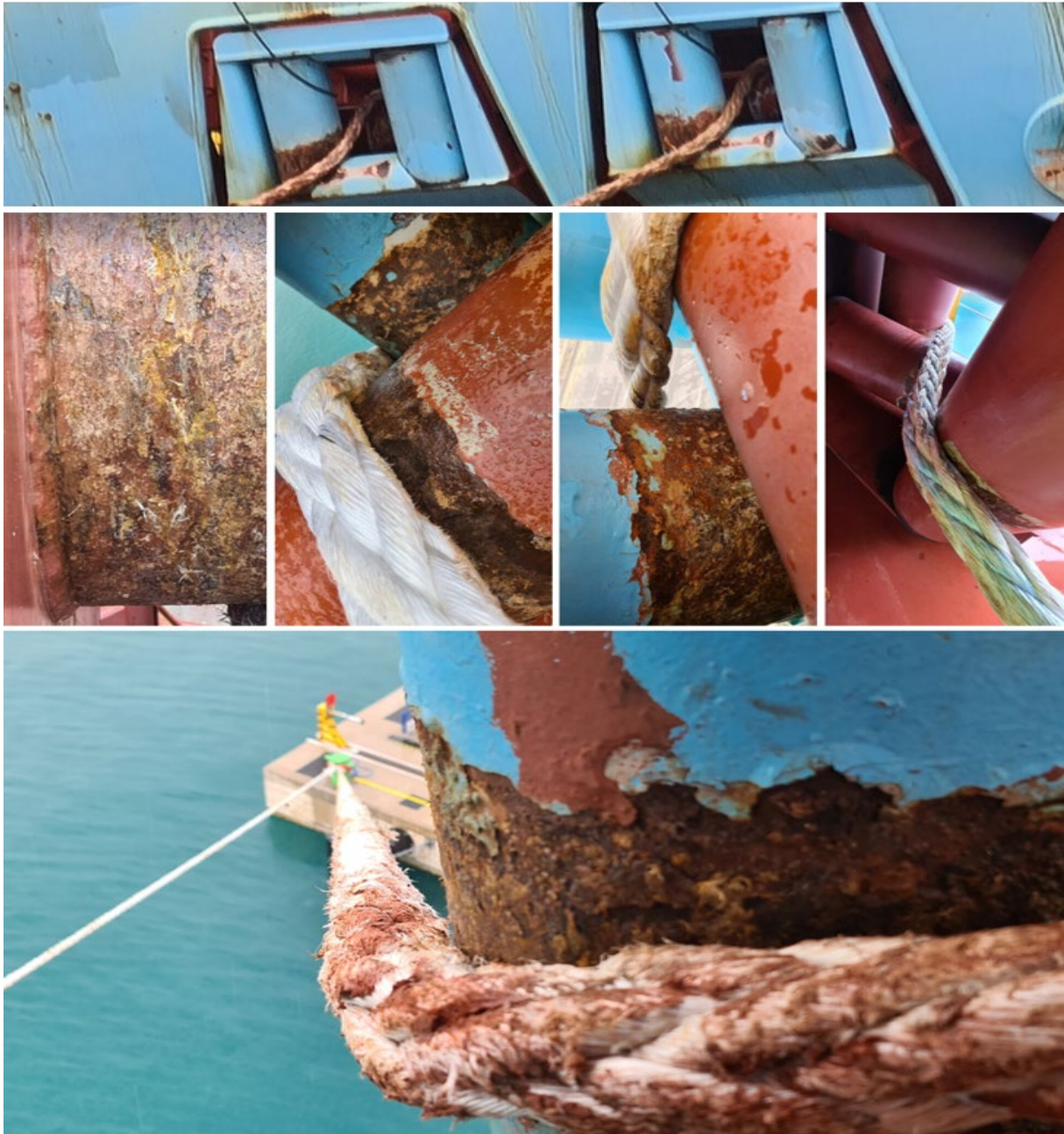
Figure 25: Inspection of ropes and guides, showing corrosion of mooring equipment
