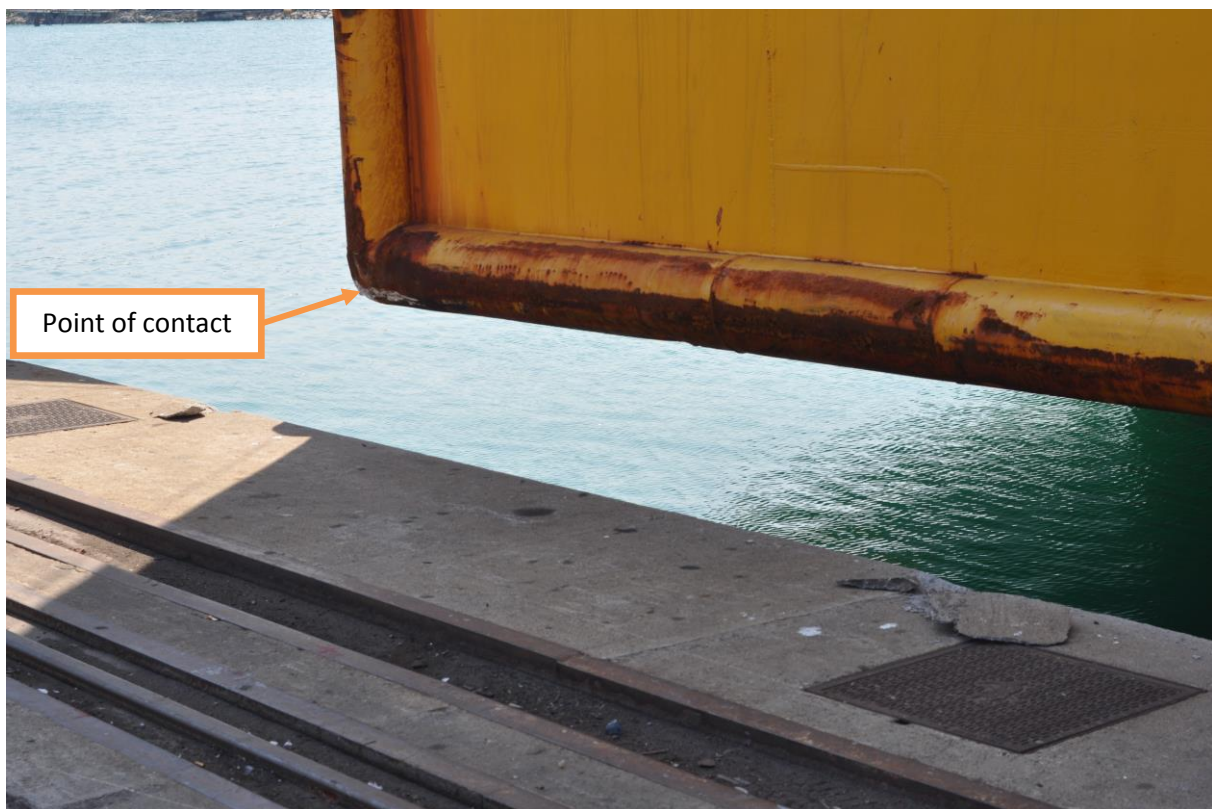
Picture 3: Point of contact, ship’s stern starboard side
