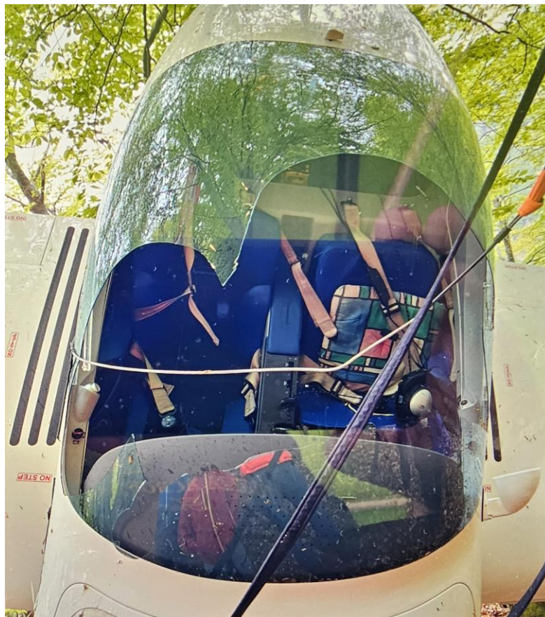
Figure 7: D-MSHU at the occurrence site with fractured front canopy
