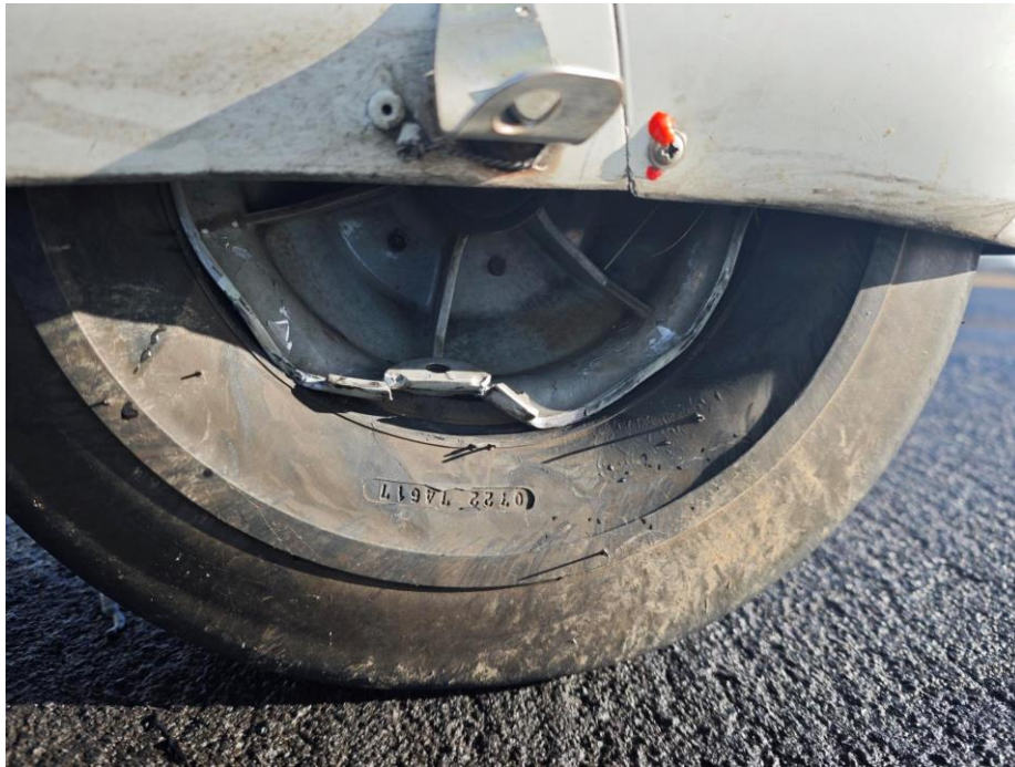
Figure 3: Aircraft damage - nose wheel
