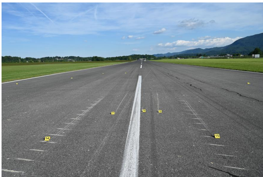
Figure 3: OE-FPV - propeller strike marks on the runway during the take-off phase
