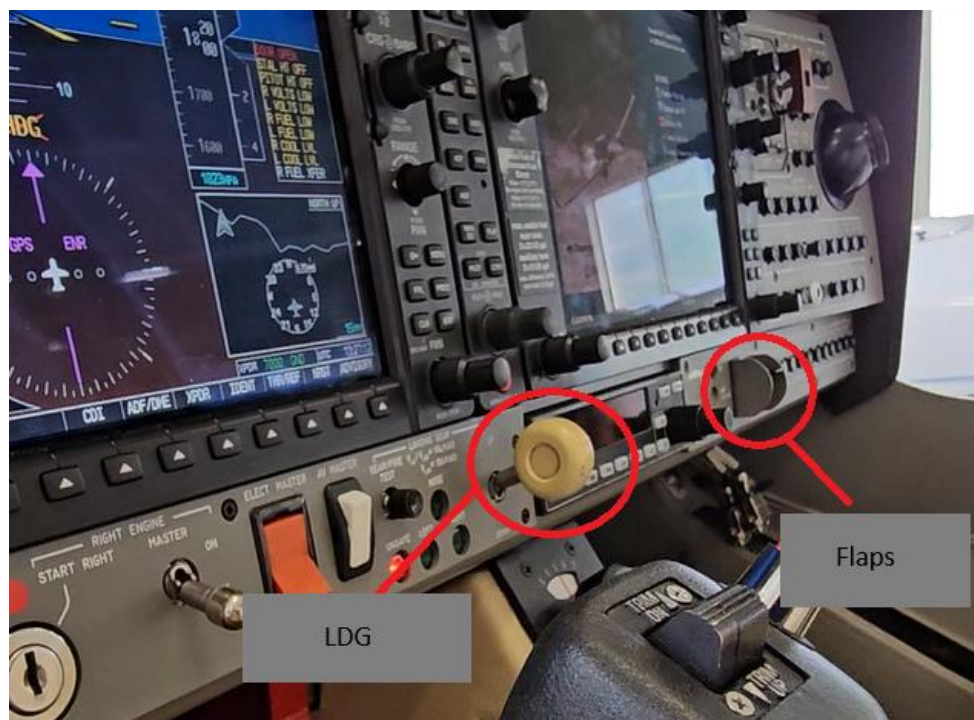
Figure 4: OE-FPV - position of configuration control levers: left - LDG, right - Flaps
