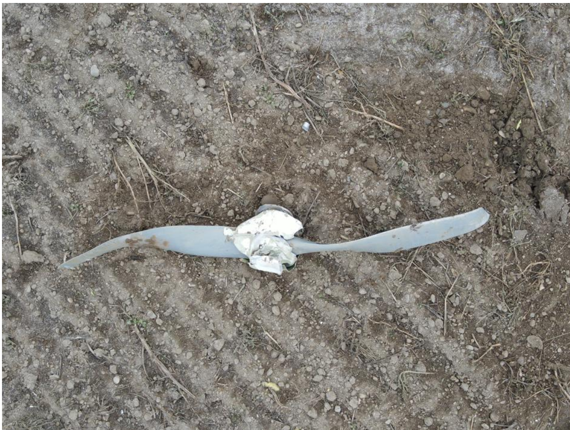
Figure 2: Fractured propeller blades at the accident site
