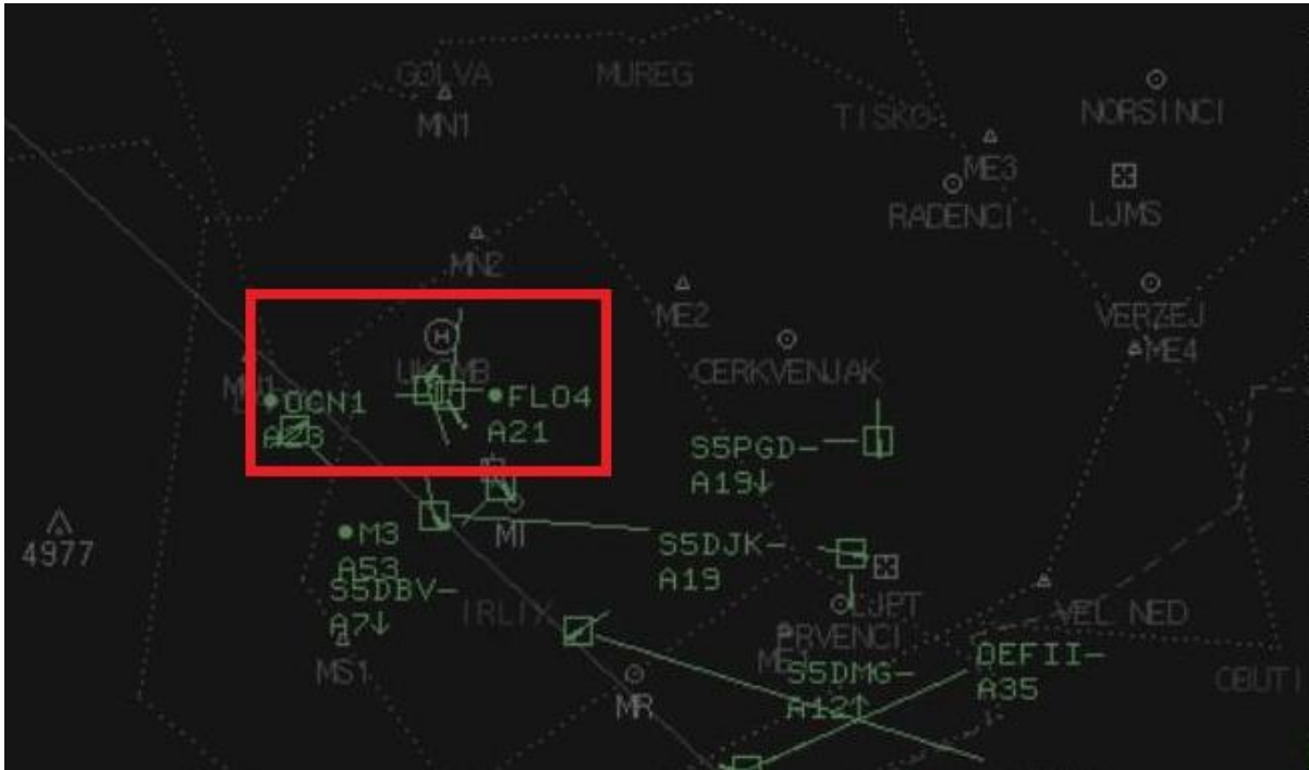
Figure 2: Radar display of traffic within the Maribor CTR at the time of the airprox between the aircraft (OCN1) and the helicopter (FL04)
