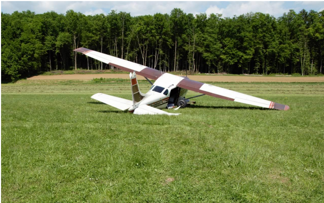
Figure 1: Aircraft position following the failure of the right main gear spring leg
