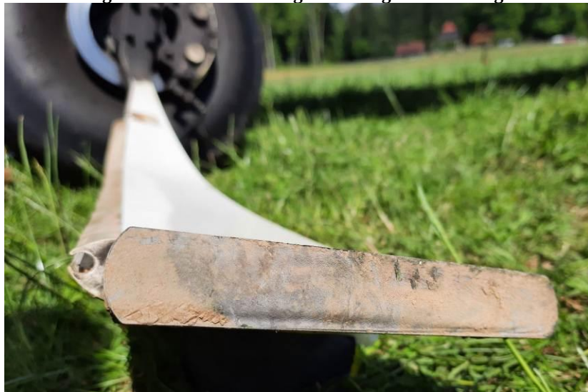
Figure 8: Detached spring leg section found on the grass
