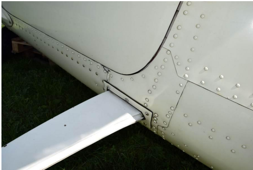
Figure 6: Spring leg entry point into the fuselage
