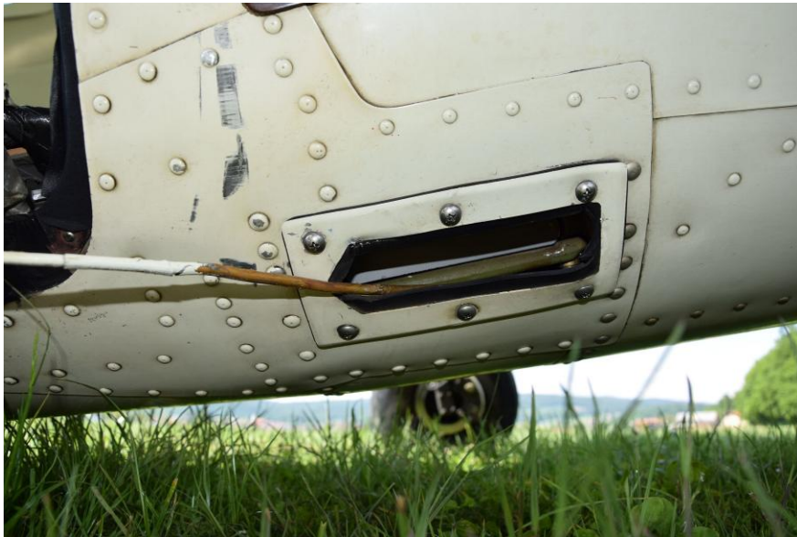
Figure 7: Section of the leg remaining in the fuselage
