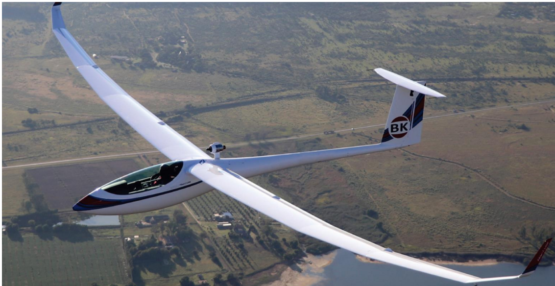
Figure 2: Jonker JS-MD 3 glider with auxiliary JET engine
