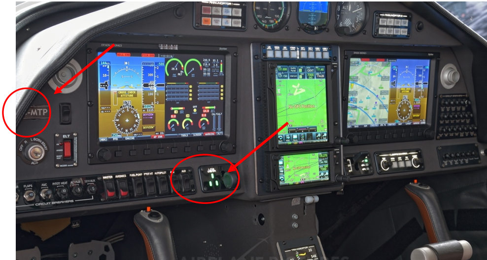
Image 2: Position of the LDG selector switch on Panthera registered S5-MTP
