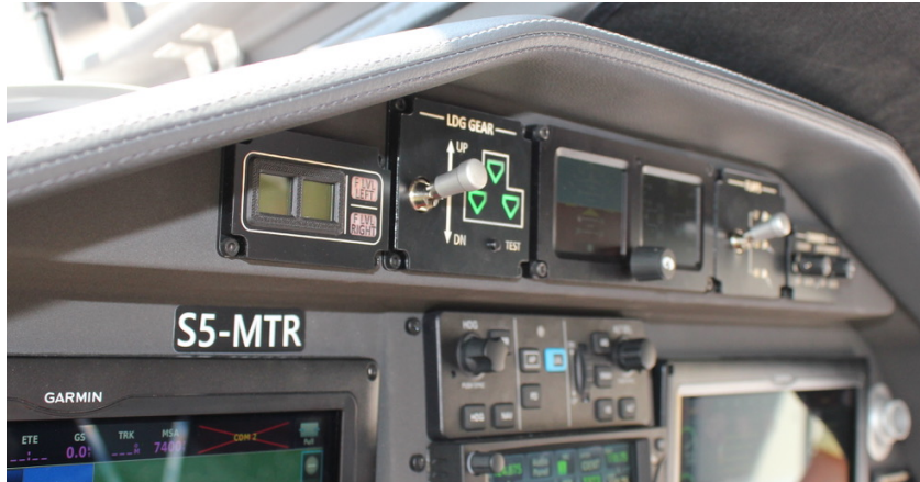
Image 4: LDG selector switch position and light signaling after landing gear emergency extension
