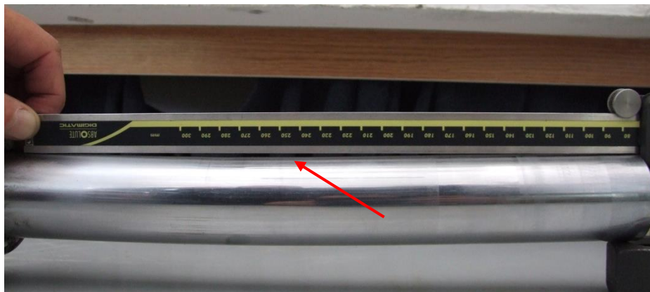
Figure 16 Bent piston of the left LDG leg shock absorber
