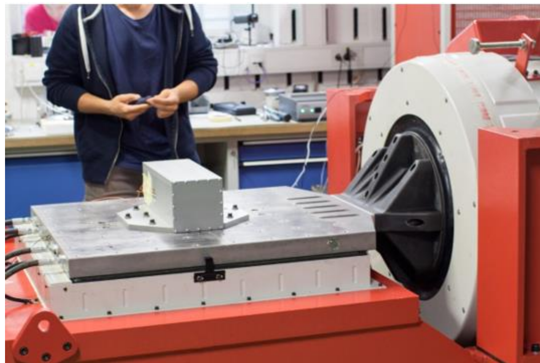
TRISAT vibration test fixture mounted on slip table for mechanical and environmental tests.
