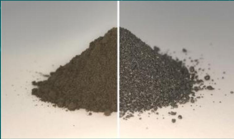
◀ **Space Resources:** 'before and after' demonstration of oxygen and titanium extraction from lunar regolith simulant using Metalysis process
