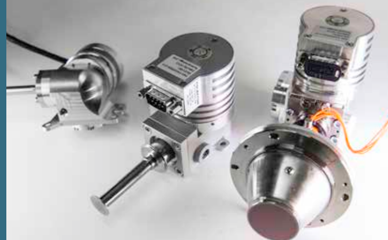
Miniature rotary Stirling cryocoolers with cooling powers from 0.25W to 1W at 77K
