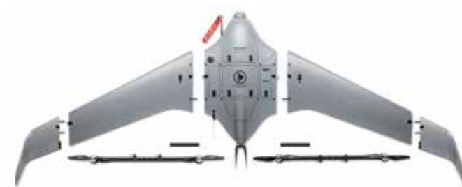
SQA eVTOL Unmanned Aircraft System modular assembly view with main components (C-Astral SQA unmanned system 6)
