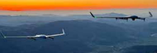
SQA eVTOL Unmanned Aircraft System in flight – left with nose mount gimbal, right with belly mount gimbal camera (C-Astral SQA unmanned system 2)
