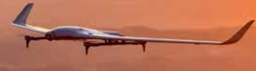
SQA eVTOL Unmanned Aircraft System in flight – left with nose mount gimbal, right with belly mount gimbal camera (C-Astral SQA unmanned system 2)
