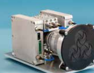
2U GEO redundant Transponder Telecommunication Payload
